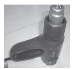
Please note this tool no need any lubricant and grease to use for inside components.
